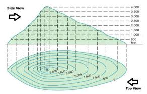
Within contour lines there is something called a contour interval (CI) which is the distance between contour lines. The CI value is usually shown on the lower part of the map or can be easily calculated using the index lines. The index lines are the thicker brown lines that give you the actual elevation above sea level for that specific contour line. Index lines are usually every fifth line on a topographical map.
